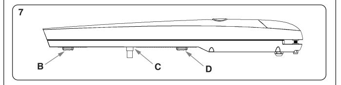
① The gear-motor are manually provided with mechanical stops in open position. In case of lack of external mechanical stops in closing position, it is possible to buy the optional mechanical limit switch.
