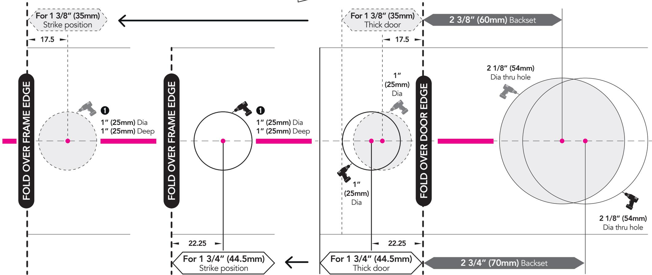
**!** Check the deadbolt and strike positions center before drilling
