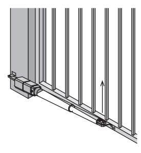
Remove the spring clip and pull the manual release clevis pin
