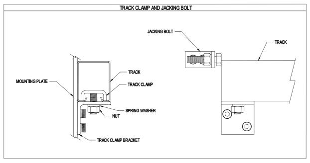
Ensure that the jacking bolt is fully tightened into its bracket. Push the non-idler end of the track over the track clamp which fits over the internal lips of the track. Push the track over the clamp until its edge touches the head of the jacking bolt as below.
