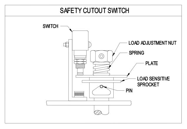
The Safety Cutout Switch is designed to protect the door against severe collision during operation. If the door is obstructed the unit will keep trying to move the door until it reaches a torque set by you. At this torque, the Load Sensitive Sprocket will depress the Switch.
