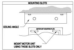
When fitting the motor unit to the angle bracket, you should avoid over tightening the mounting bolts. Nyloc nuts should be tightened only slightly firm, enough to remove any play or slop. It is recommended that a Loctite thread adhesive be used. If vibration is still evident, loosen the mounting bolts.
