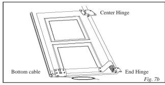
**Step 8** As each door section is completed, the rollers must be placed in the brackets and hinges as shown in Fig. 8. Once complete slide bottom panel into vertical tracks, (refer Fig. 9), ensure rollers are engage in track and moving freely.
