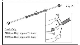
Once you have completed the desired number of turns secure the set screws on the spring block to the shaft. Remove the winding bars.
