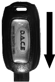
Step 5: Insert D.B.C into pins labelled DIGITAL B/CARD
