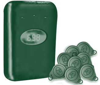
Access control proximity unit
