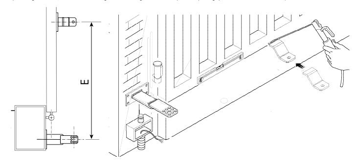
Fasten the gearmotor to the braces by using the supplied nuts and bolts.
