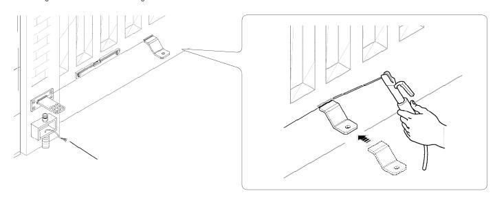
On non-metallic leaves, assemble and weld the two parts of the brace - use suitable screws to fasten.
