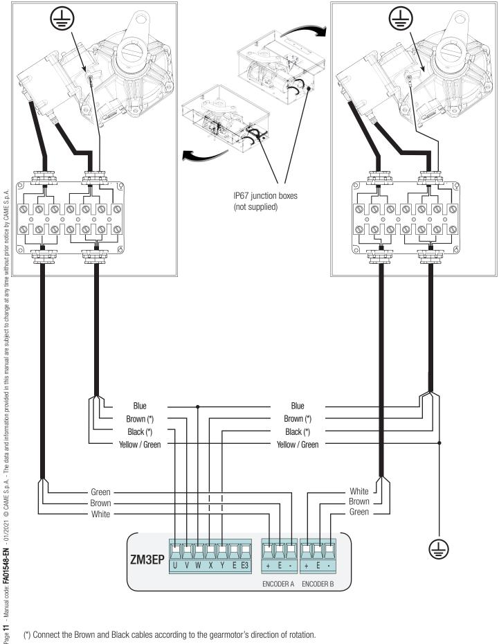
(\*) Connect the Brown and Black cables according to the gearmotor's direction of rotation.
