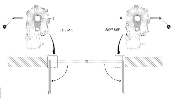
Open the door to facilitate the placement of the gearmotor in the foundation case and its anchoring. Secure the gearmotor using the nuts supplied.
