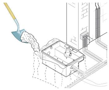
Position the box level with the ground and place the pin in line with the upper gate hinge. Leave to solidify for at least 24 hours. Clean any remaining concrete from inside the box.
