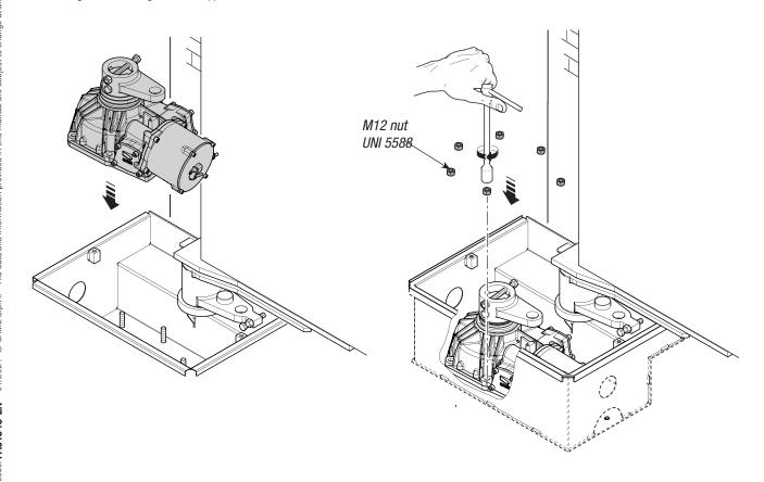
Lubricate the transmission lever and fit it into the hole of the gearmotor arm and case lever.
