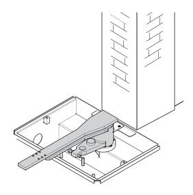
Install the gate leaf, inserting the upper hinge. Fix or carefully weld the leaf to the fixing bracket to the gate. Check that the leaf opens and closes without difficulty.
