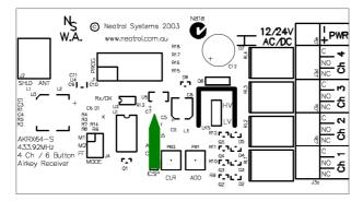
The remote learning socket must be removed before connecting an Airkey Programmer, Airkey Manager or using the manual ADD or CLEAR buttons.
