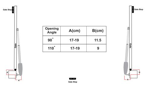
Gates Open in a Push to Open Installation
