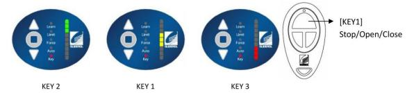
**Three Button Configuration:** Each buttons in the transmitter can be used to control individual functions like functions Stop/Open/Close of eth same door.
