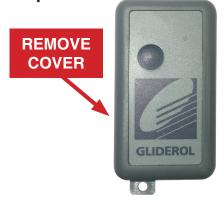
Remove the cover from the handset to expose the handset circuit board.
