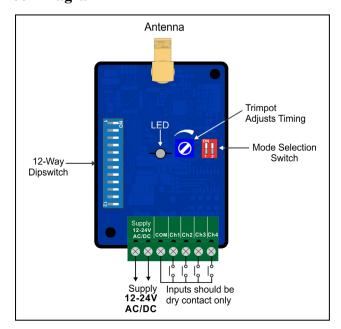
Inputs of the transmitter should be voltage free contact closure only.
