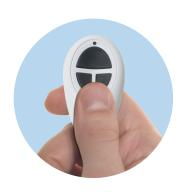
Press the button on the handset that you would like to operate the door. The unit will beep once to confirm successful coding (two beeps indicates the handset has already been programmed). Wait approx 3 seconds for the unit to exit setup mode.
