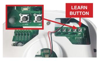
Press the 'Learn' button once. A red light will illuminate and the unit will beep three times to confirm the unit is in learn mode.
