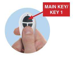
Press the Main/Key 1 button on the handset. The unit will beep twice to confirm successful coding. Wait approx 3 seconds for the unit to exit setup mode.
