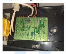
3. Remove the receiver from the wall panel to expose the backside and gain access to the SW1 button circled below.
