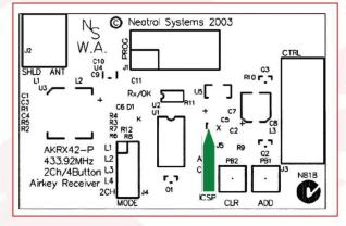
other peripherals. The learning socket should be fitted when power to the receiver has been disconnected. If this is not convenient, simply press and hold the ADD button while carefully installing the remote programming socket. Local programming with the remote learning socket removed Before any transmitters are learnt into the receiver for the first time, press and hold the CLR button on the receiver for about
