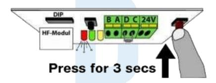
3. On the new remote, press and hold any button that you wish to operate the door. The LED on the motor should stop flashing after1-2 seconds once the remote has been programmed.
