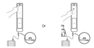
To open the door, connect a Micro USB 5-Pin cable from a smartphone portable charger to the Micro USB power input on the bottom of the outer body, and then authenticate the fingerprint or enter the password.
